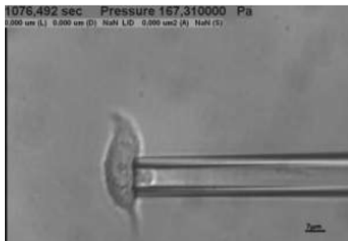
Fig.1 Adhered breast cancer cell (MCF-7) deforms via micropipette aspiration technique.
